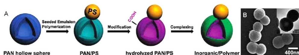
Figure 1. (A) Schematic illustration of the preparation of Janus PAN/PS colloidal particles via the seeded emulsion polymerization of St in the presence of cross-linked PAN hollow seed, followed by PS bulge growth on seed particle and favorable growth of other materials, (B) Scanning electron microscopy (SEM) of Janus PAN/PS polymer colloidal particles (monomer/PAN seed weight ratio = 4:1 with the DVB/St weight ratio at 3:1). Reproduced with permission from ref 14. Copyright 2010 American Chemical Society.
